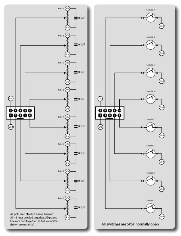
\* Please note that connection to +5V is not necessary for any SPST switch.
